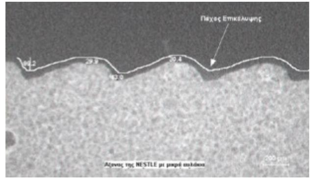
Figure 14. Wear Coatings on Coffee Mill Rolls - HVOF, Carbide Coating
