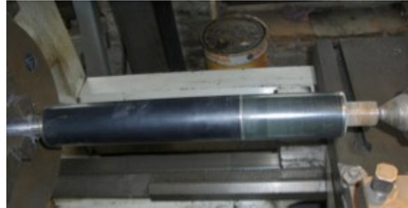
Figure 15. Wear Coating and Restoration of Hydraulic Systems - Plasma Spray, Ceramic Chrome Oxide
