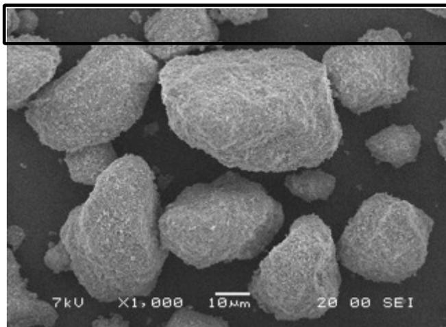
Figure 9. Agglomerated nanostructured particles before thermal spray
