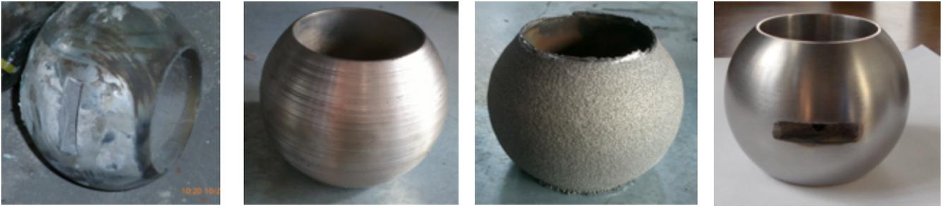
Figure 10. Restoration and Wear Coating of Valve Ball - Flame Spray, Hard Steel Coating
