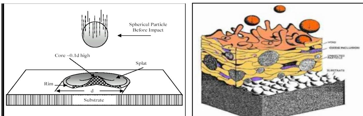
Figure 1. Schematic diagram of spherical particle impinging onto a flat substrate (left) and 3D view of deposited coating (right)
