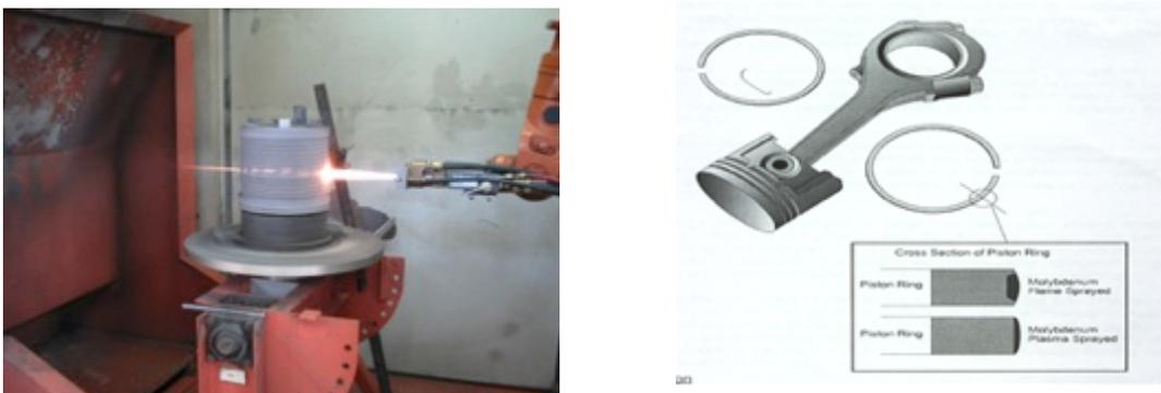
Figure 13. Friction-Wear Coatings on Piston Rings - HVOF, Carbide Coating
