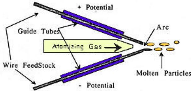
Figure 5. Wire Arc Spray process:
