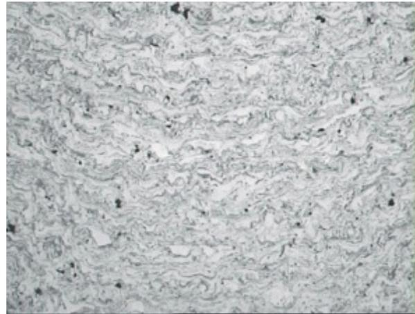
Figure 8. Flame spray Fe-based coating with 20-25% oxide content
