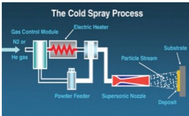
Figure 6. Cold Spray process:
