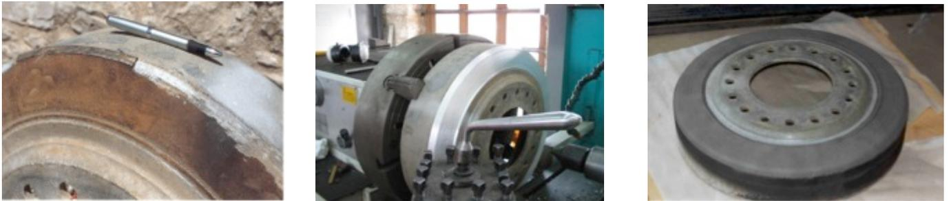
Figure 11. Restoration and Wear Coating of Army Tank Al Wheels - Wire Arc Spray, Hard Steel Coating
