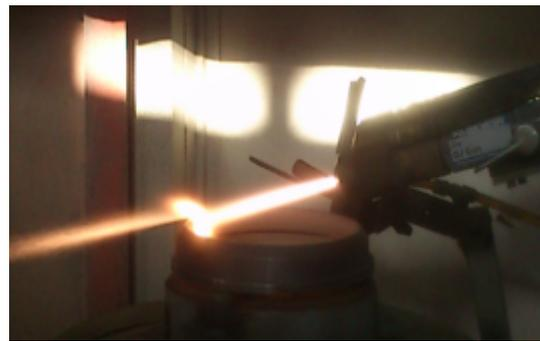
Figure 16. Wear Resistant Coating on Turbocharger Nozzles - HVOF, Carbide Coating
