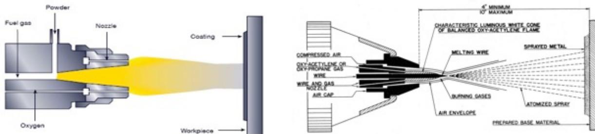
Figure 4. Flame Spray process: (a) powders, (b) wire
